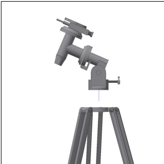
Figure 4. Place equatorial head on top of tripod..
