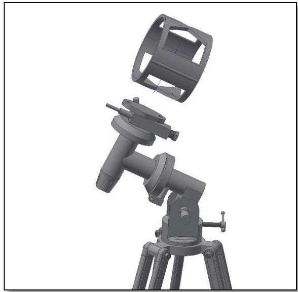
Figure 5. Place the tube rings.
